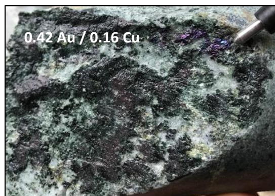
EPDD001 320m. Coarse-grained bornite along shear zone + actinolite.
