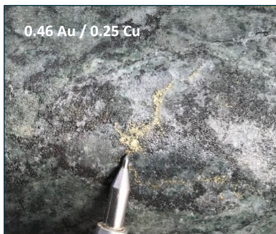
EPDD001 225.8m. Quartz-magnetite-chalcopyrite vein in quartz-chlorite-magnetite-actinolite-epidote-calcite altered porphyry
